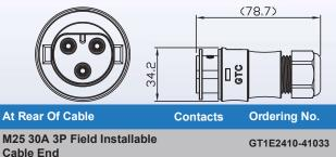
(88.2) N 12 Щ 34. At Rear Of Cable Ordering No. Contacts M25 30A 3P Field Installable
